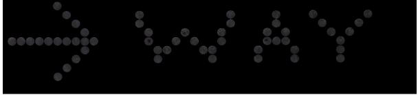
Figure 1.7 Lines and text on a point-plotting display, enlarged to show individual pixels
