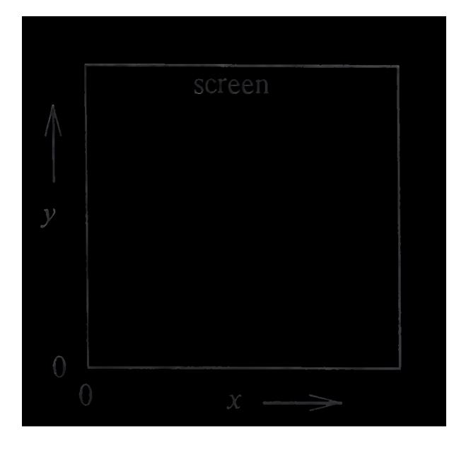
Points are plotted in response to digital signals from the computer. This means that they cannot be positioned with infinite precision; instead we are limited by the precision of the digital values presented to the display. For example, if x and y are passed to the display each as a 10-bit binary number, there can be only  $1024 (= 2^{10})$  distinct x-coordinate values and only 1024 for y. The screen offers us a 1024 X 1024 array of positions, at any one of which a dot may be displayed.
